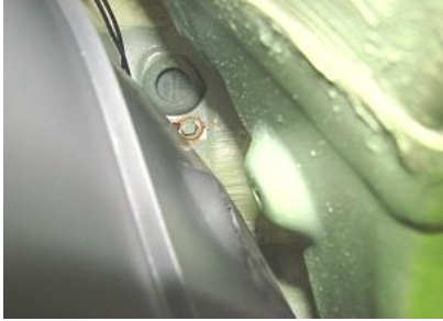
G204 (below right pillar C)
