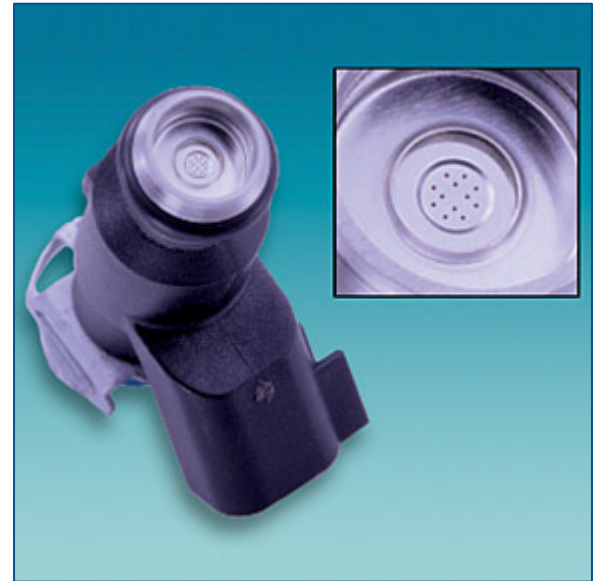
The tip of Delphi Multec® 3.5 Fuel Injectors features a multi-hole director plate that provides fine atomization.
